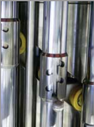
Upper plunger spring compression adjustment
