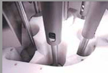
Dual turret "Slide Fill" style fill basin
