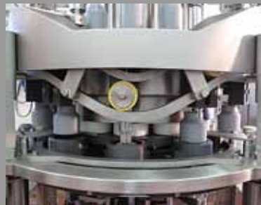
Single turret - product discharge area
